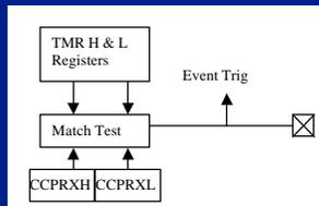
CCPx pin toggle event is driven by the match of a moving 16 bit counter, timer 1, against a known 16 bit value, cascaded CCPRxH and CCPxL value. When timer 1 equals CCPRx, a CCPx bit toggles, an interrupt or special event trigger occurs. The special event trigger output of CCP will cause a reset of timer 1 high and low bytes, and offer a means to start a conversion cycle in many mid-range parts containing an ADC module.
