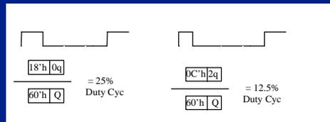
Conceptually, the proportional percentage of the duty cycle output is reflected by CCPxL to PR2.
