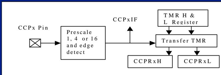
The capture mode functional diagram illustrates how the incoming pulses are divided by the pre-scaler value before setting the CCPxIF flag, indicating a positive capture condition/event. The signal evaluated by the pre-scaler originates from the external CCPx pin and routed to the pre-scale circuitry. A pre-scaler is used to increase the number of edge counts required before sending the CCPxIF and transferring Timer high and low contents to CCPRxH and CCPRxL registers.
