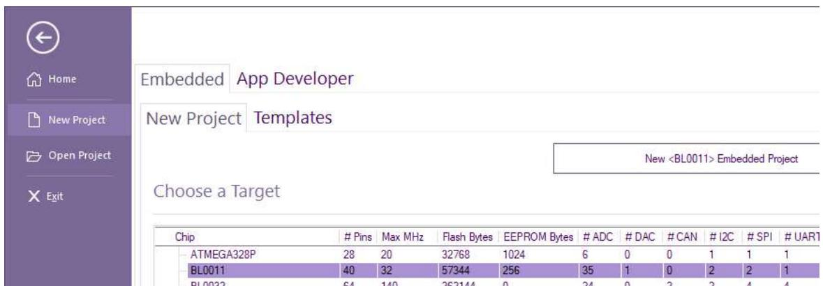
In this case the target choice also selects the correct 16F18877 device and presets the correct values for clock oscillator frequency and other settings.
