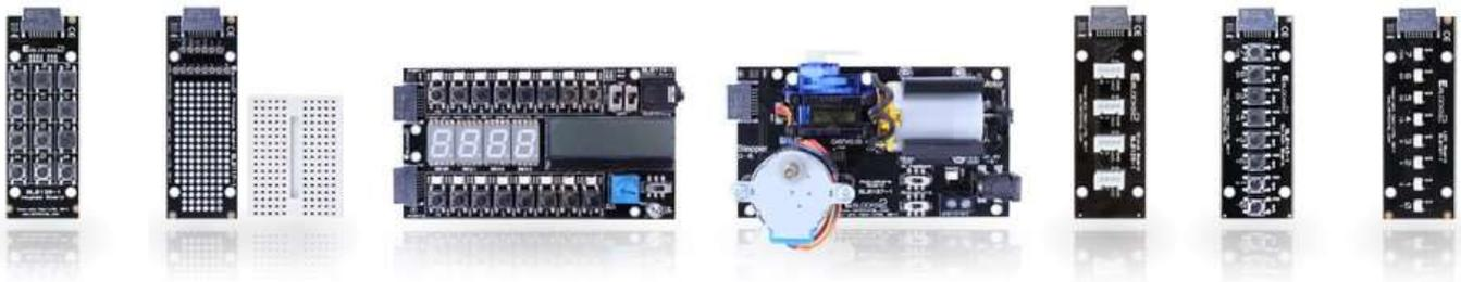
*Upstream and downstream boards combined to form a full system, with the downstream boards plugging into the upstream 'intelligent' boards:*
